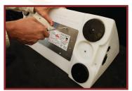
Plug new light panel into the pig-tail located inside of the sign. With the anchors in place and expanded, replace panel over the opening, aligning the pre-cut holes with anchors and secure to the sign with screws.
