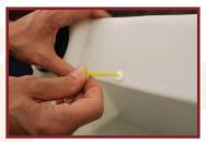
Fold the wings of the anchor completely inward and insert into the drilled hole until flush. Insert the yellow pin into the anchor to expand anchor wings inside of the sign.
